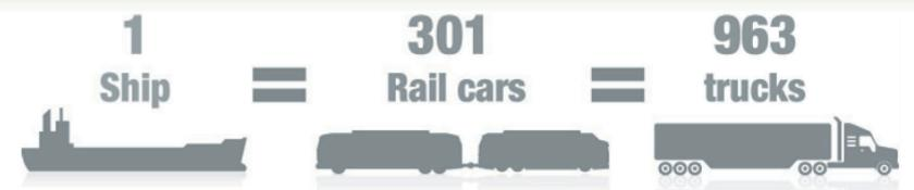
Based on the maximum carrying capacity of Seaway-size vessel
